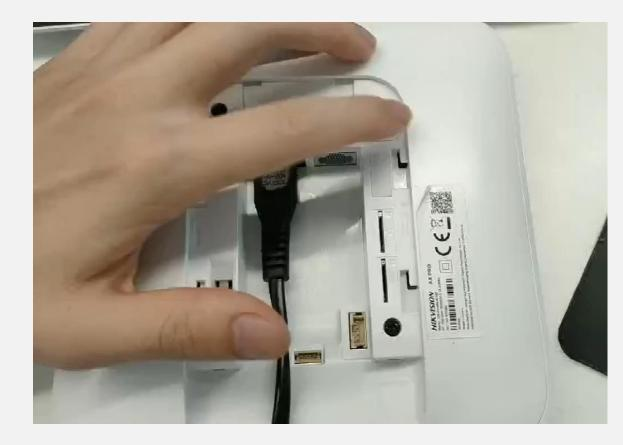
Power on the hub, when hear the first voice, press and hold on the reset button
