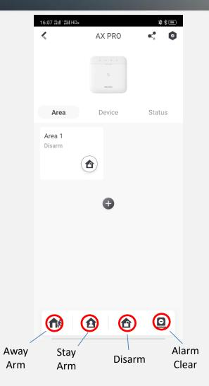
These four buttons are used for the whole system, not for a single area.
