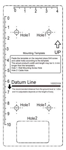
**Figure 3-4 Mounting Template**
