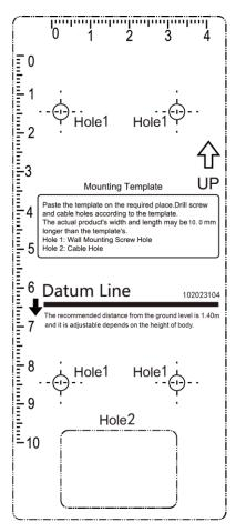
Figure 3-2 Mounting Template
