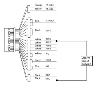
Figure 2-5 Alarm Input Device Wiring
