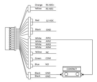
Figure 2-3 Door Contact Wiring
