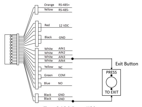
Figure 2-4 Exit Botton Wiring
