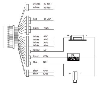
Figure 2-2 Door Lock Wiring
