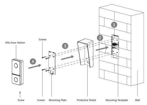
Figure 3-5 Flush Mounting with Protective Shield
