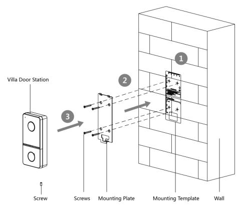
Figure 3-3 Surface Mounting without Protective Shield
